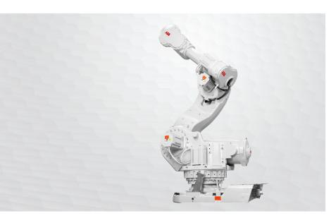
With several variants, and up to a 630 kg handling capacity, the IRB 7600 is ideal for weighty applications, regardless of your industry. Characteristics such as high available torque and inertia capability, rigid design, and powerful acceleration have earned this market leader its "Power Robot" title.
