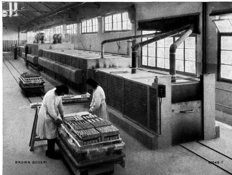
Fig. 81. — Single electric tunnel kiln for the firing of steatite at 1400^{\circ}\text{C} . First electric tunnel kiln for firing of steatite.
