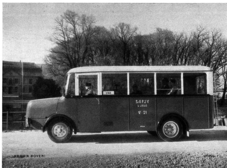
Fig. 109. — Bus owned by the S. A. des Autotransports du Pied du Jura Vaudois, L'Isle (Switzerland), with Saurer chassis and Eggli coachwork, for battery operation.
