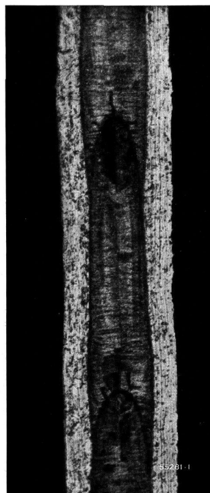
Fig. 77. — Ground section through seam weld of two stainless steel sheets 0.08 mm thick. Frequency of individual spots 200/sec. without interruption.
