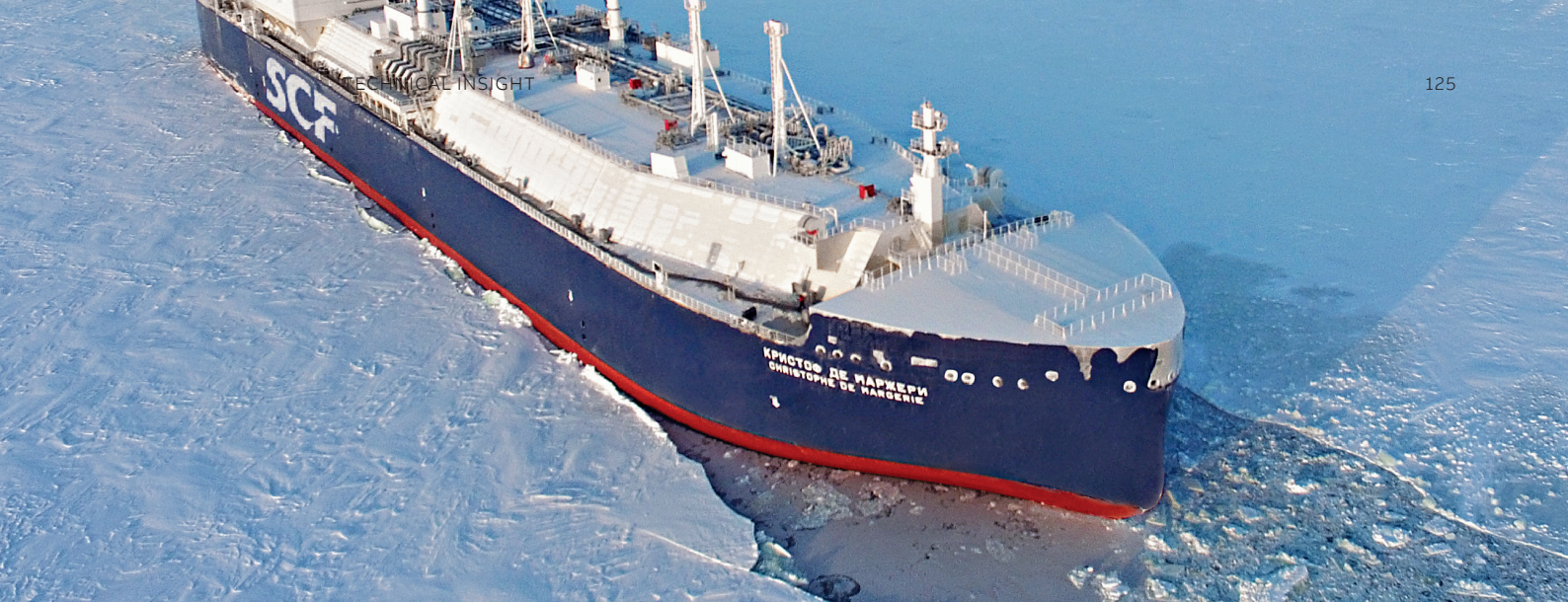
Figure 1 (over): SCF – Sovcomflot IMO 9737187 Christophe de Margerie (previously DSME H2418), the world's first Yamalmax electrical propulsion LNG carrier with ARC-7 ice class
