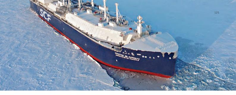
Figure 1 (over): SCF – Sovcomflot IMO 9737187 Christophe de Margerie (previously DSME H2418), the world's first Yamalmax electrical propulsion LNG carrier with ARC-7 ice class
