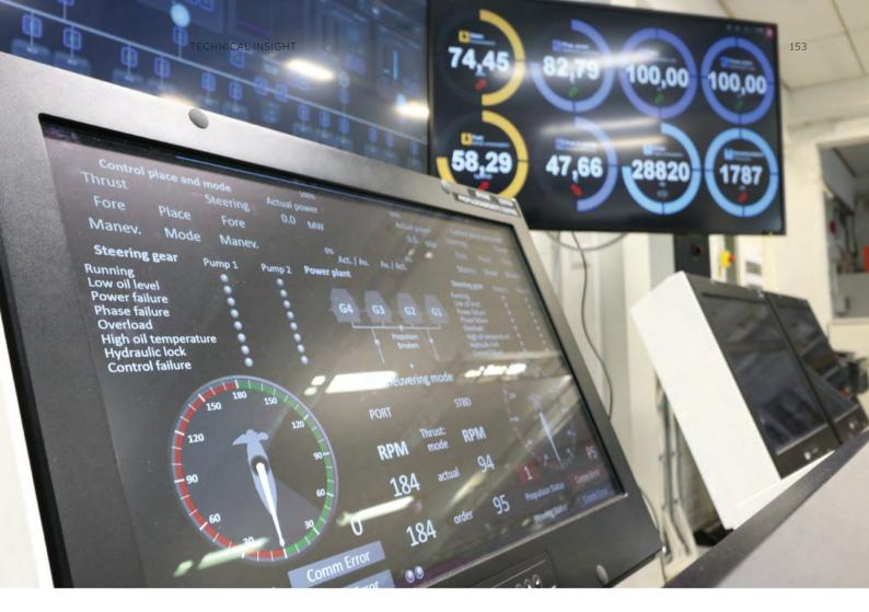
Figure 1: A section of the Integrated Marine Systems Laboratory. The lab consists of the pillars of ABB's marine technologies including automation, remote control systems, propulsion, integrated operations and waste heat recovery systems.
