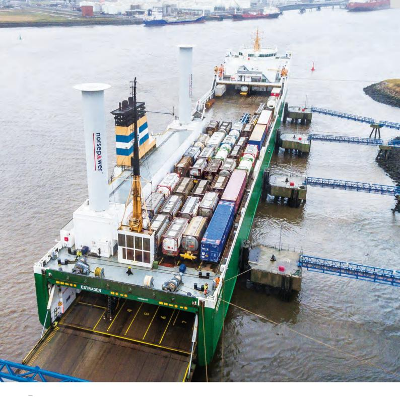
The sail is rotated using electric power, but energy consumption is low, enabling the sail to provide a propulsive thrust in favourable wind conditions equivalent to more than 10 times the propulsion shaft power than it consumes. With the addition of Norsepower's technology, the LNG-fuelled Viking Grace will further reduce its emissions, fuel burn, and fuel costs, reducing carbon emissions by approximately 900 tonnes annually, or the equivalent of 300 tonnes of LNG fuel each year.
