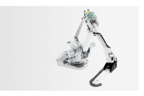
The benefits of traditional robot automation are enhanced by the addition of a rotational 7th axis. Thanks to 7th axis, the robot keeps the orientation of the part when transferring it from a press to the next. This entails lower inside-press time occupation and better overlapping between loading and unloading robots.
