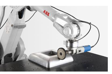
Integrated Force Control is one of the key technologies driving the uptake of industrial robots. ABB's Integrated Force Control function facilitates the ease-ofuse for robots in applications requiring real-time adaptive motion control.
