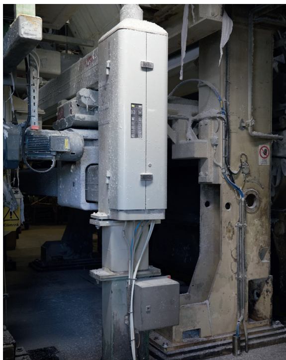
Two sensors measuring moisture and fiber weight have been replaced with the infrared (IR)-based HPIR-FW sensor in PM8 at Lilla Edet's tissue paper mill.
