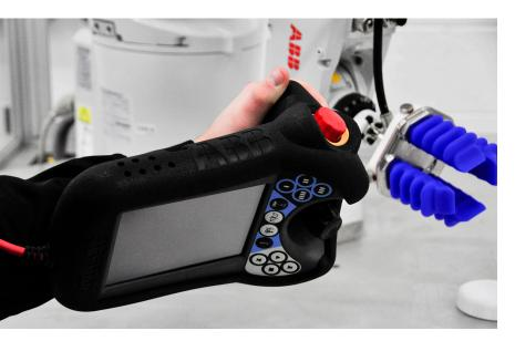
The ABB IRC5 FlexPendant Protective Bumper provides added protection if the FlexPendant is accidentally dropped.
