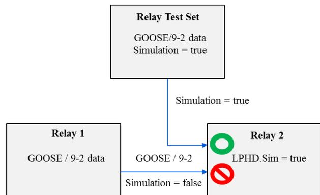
Figure 2. Simulation according IEC 61850
