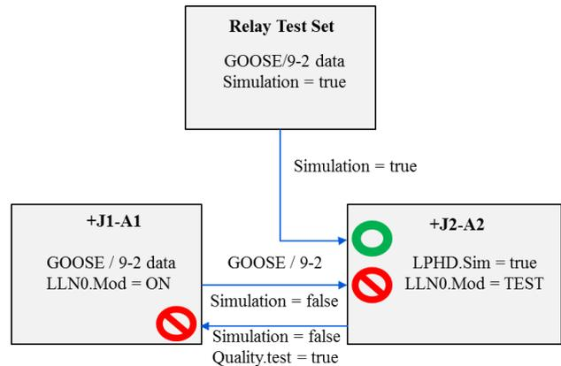
Figure 5. Periodical testing connecting relay test set to IEC 61850 communication bus
