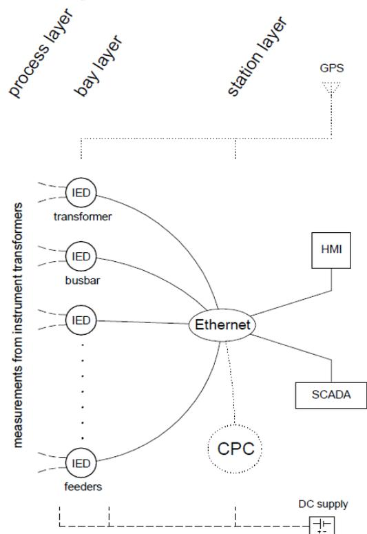
**Fig. 1.** Schematic of the Block-layer reliability technique adjusted to secondary substation systems connected to the process level (left) and to adjacent substations (right). Time-synchronization sources (GPS) and DC supplies are parallel components, crossing several layers, consequently they are not included to any layer.
