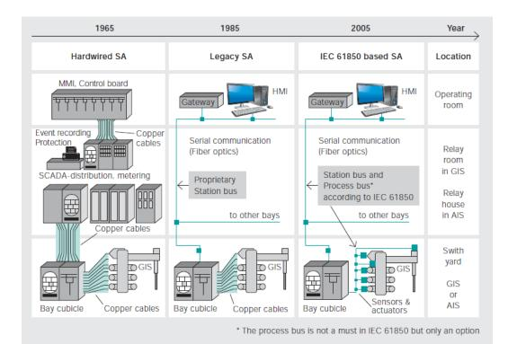
Fig. 2 Secondary substation system in the three levels (process, bay and station levels from bottom to top) in three different stages: hardwired, Legacy and IEC 61850-based systems [7].
