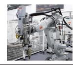
RobotWare-Dispense can be used for different types of dispensing processes. It is a software option typically used for gluing, sealing, spraying and other similar processes, but can also be useful in a wide spectrum of other applications.
