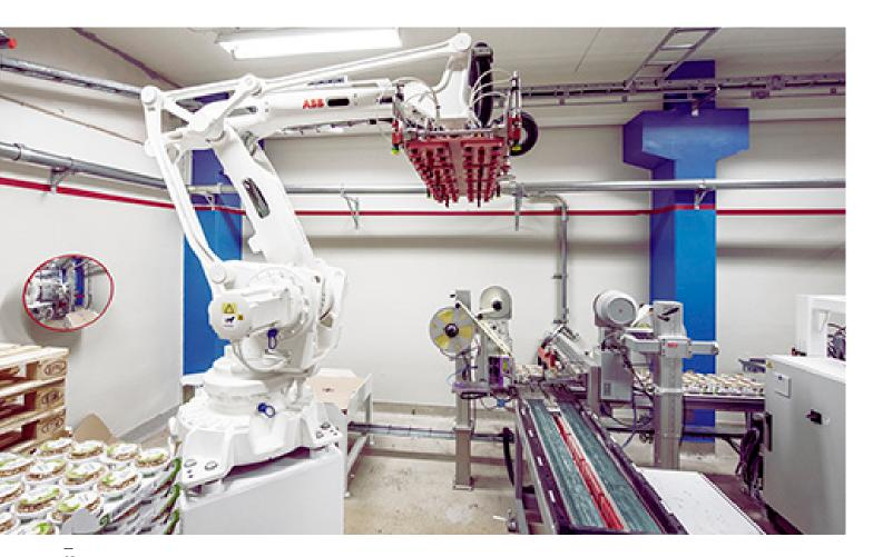
The four-axis IRB 460 can lift 48 containers with their tray at a time, then stack the trays on the pallet with millimeter precision. One pallet fills in 10 mins, corresponding to a total of 8,500 products an hour.
