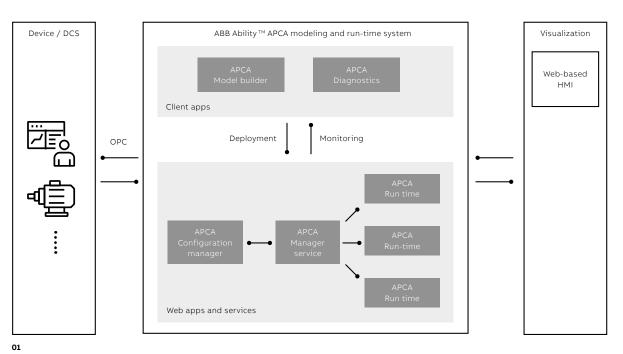
Currently, the ABB Ability<sup>™</sup> Platform is the digitally enabling technology that allows the implementation of APC solutions.
