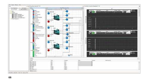
The predictive power plant optimization solution uses the predicted power demand of a ship during its entire voyage as input data, which is then exploited to determine the optimal load for each generator.
