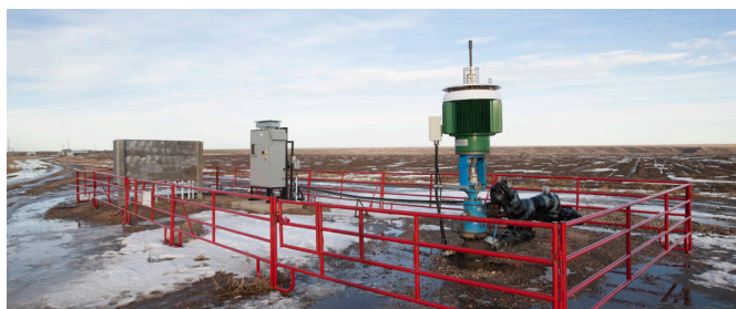
Figure 3. Variable speed drives can help optimise the production according to the changing well conditions and protect both the equipment and the people using it.
