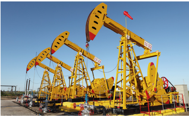
Figure 1. Connecting artificial lift systems to digital communication networks and using real time data from variable speed drives and sensors helps to significantly increase production rates and reduce downtime.
