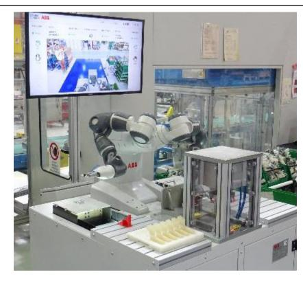
ABB robot YuMi with Artificial Intelligence application that allows the robot to be operate via gesture
