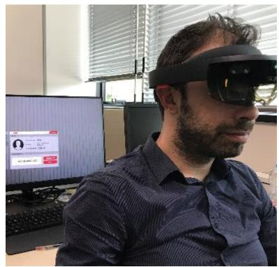
ABB worker wearing Hololens will look at the equipment during assembly. The system with identify the QR code and will automatically propose the next assembly stage.
