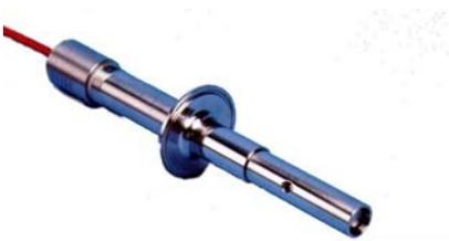
*TB25 is a sterilizable 2-electrode stainless steel body conductivity sensor. It is often used on measuring rinse water conductivity.*
