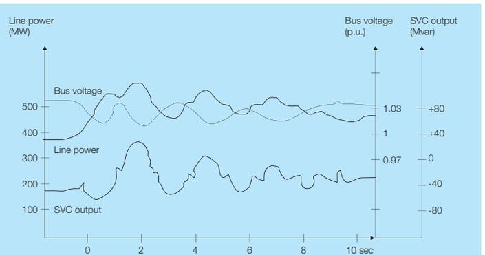
Damping of power oscillation upon trip of a 100 MW generator unit. Oscillation damped out after 9 seconds. Maximum 330 kV voltage deviation during POD: 2,7%
