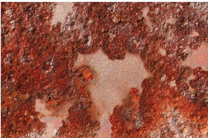
In its dissolved form, oxygen is highly corrosive to most metals, especially the mild steel used for boiler tubes.
