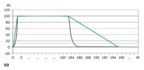
The new version of the ABB TZIDC positioner Rev. 3.00 now allows for the combination of a set point ramp with a control characteristic. This type of set point processing is in no way a state-of-art solution for 4 to 20 mA devices.
