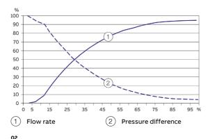
Quite critical are ranges < 15 %, in which nearly 50 % of the mass flow needs to be decelerated with less than a fifth of the opening cross-section. The state-of-the-art approach is to close pipes, flanges and valves with the risk of developing water hammers in a controlled manner using mechanic-pneumatic devices or electric multi-turn actuators, whereby additional pipe protection
