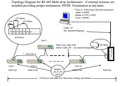
Figure 9 - Termination Using External Resistors On The IED's And Using The B & B Electronics Converter As An End Unit
