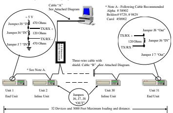
*Figure 6 – RS 485 2 Wire Termination With The RS 232/485 Converter Inline And ABB Protective Relays At End Of Line Locations.*
