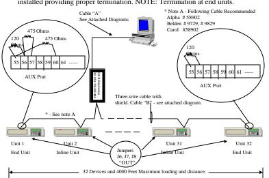
Topology Diagram for RS 485 Multi-drop Architecture - if external resistors are installed providing proper termination. NOTE: Termination at end units.
