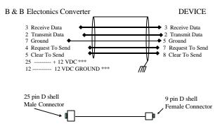
*Figure 4 – RS 232 Cable Pinout Handshaking Incorporated (See Figure 1 For Jumper Settings According To Model. DTE To DTE Connection (9 Pin To 25 Pin Rs 232 Converter Connection)*
