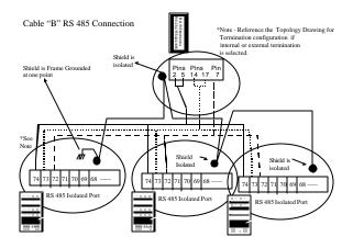
Figure 11 - Conductor Connectivity Diagram For The DPU/TPU 2000 Products
