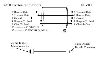
*Figure 2 – RS 232 Cable Pinout Handshaking Incorporated (See Figure 1 For Jumper Settings According To Model. DTE To DCE Connection (9 Pin To 25 Pin RS 232 Converter Connection)*
