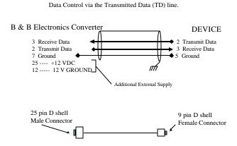
Cable "A"- RS 232 Cable for Connection from a DCE NODE and the B & B converter. NO HANDSHAKING
