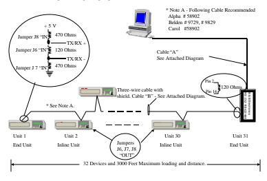
Topology Diagram for RS 485 Multi-drop Architecture - if jumpers are inserted on end units providing for proper termination and converter is at End Unit.
