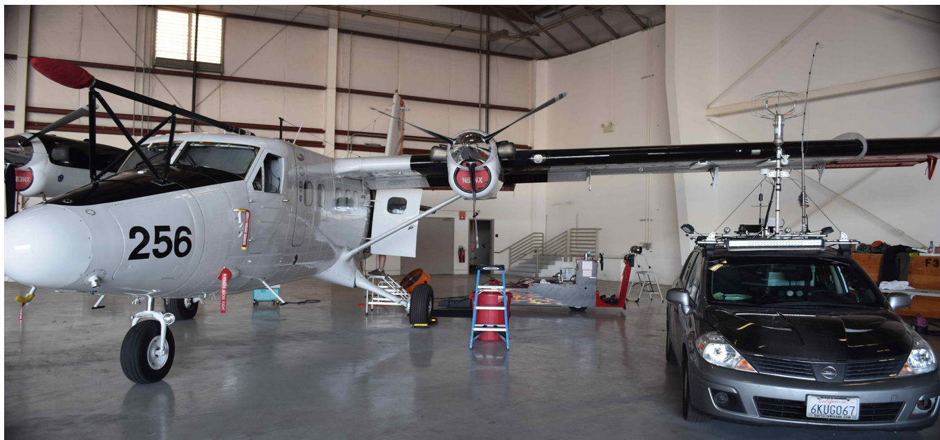
Figure. 1 COMEX instrumented Twin Otter aircraft and AMOG Surveyor
