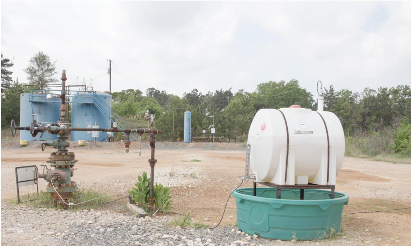
With having the output from an LST100 Ultrasonic Level Sensor input into an ABB Totalflow Control Unit (XFC or XRC), customers can monitor tank level, use rates, percent full and number of gallons in the tank, as well as able to detect refill events. The ability to monitor the level in the tank allows you to not only have an accurate inventory of what you have in the field for each tank, but gives you the information needed to set alarms, detect pump issues, monitor for leaks or theft.
