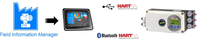
Figure. 1 The windows-based tablet with an FIM software application can replace proprietary handheld products for managing any HART instrument having an FDI device package
