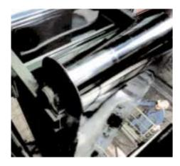
On a cold roll Cold-rolled steel is steel squeezed through powerful cylindrical rolls at room temperature to reduce thickness accurately and impart a smooth, shiny finish.
