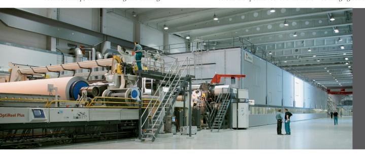
By noting both the location of the defect and the limitations of the specific winder drive the ABS calculates the optimal speed curve needed to locate the defect. It then automatically slows down the drive to either crawl speed or stop at the precise location of the selected defect. The ABS soon proved to be useful in running the winder, was told by operators.
