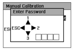
In this respect, the numbers 1, 2 and 3 are assigned to the three keys ▲, ▶ and ▼, as shown in the illustration.
