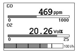
In measuring mode, the screen displays the name, the measured value in numerals and the physical unit of the measured value for each sample component.
