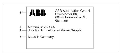
Name plate on the junction box without built-in power supply:
