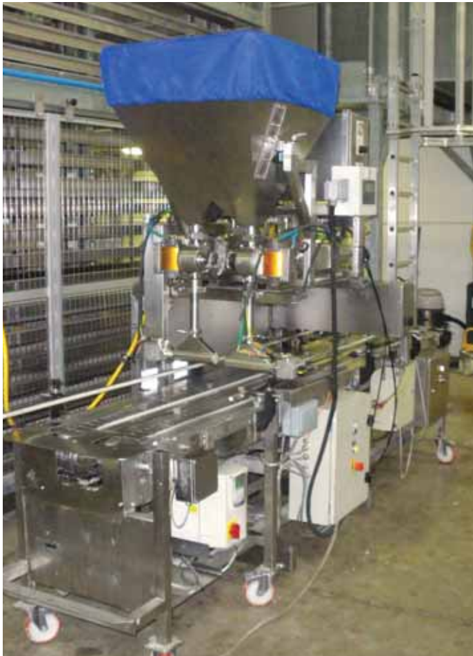
ABB machinery drive with IP66 protection class allows the bakery to be frequently hosed down.
