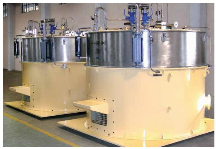
Red Sugar uses ABB general purpose drives to control the speed of the centrifuges that it assembles for the Russian sugar industry.
