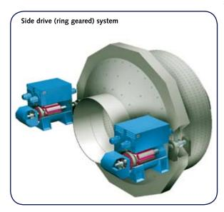
Figure 6: torque transfer happens through the pinion which inherently produces friction losses and requires regular lubrication and alignment to avoid premature failure. To run the mill at slow speeds ie, to replace liners, either a variable spped mill drive system or an additional auxiliary drive is required
