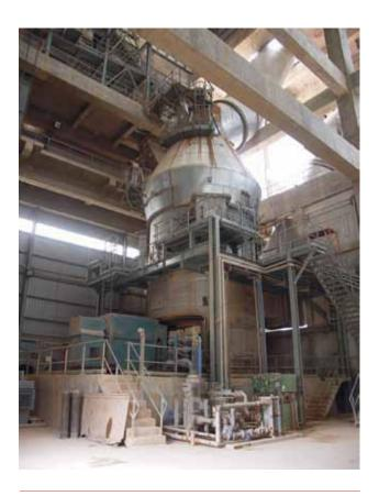
Raw mill with raw mill motor.
