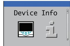
Displays read-only factory- set transmitter / wet-section details.
