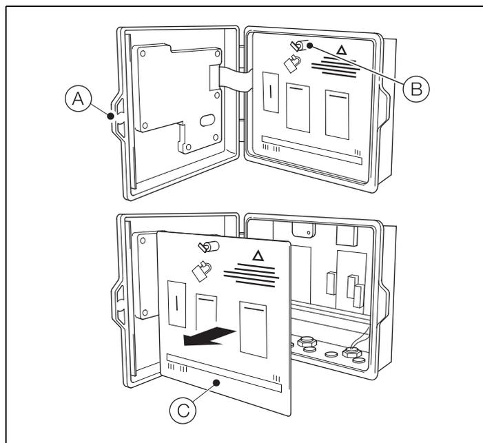
Fig. 5 Accessing the transmitter board and making electrical connections
