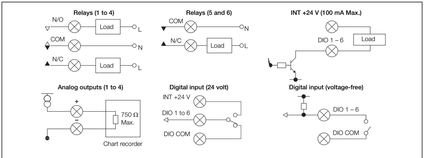
Fig. 7 Digital I/O, relays and analog output connections
