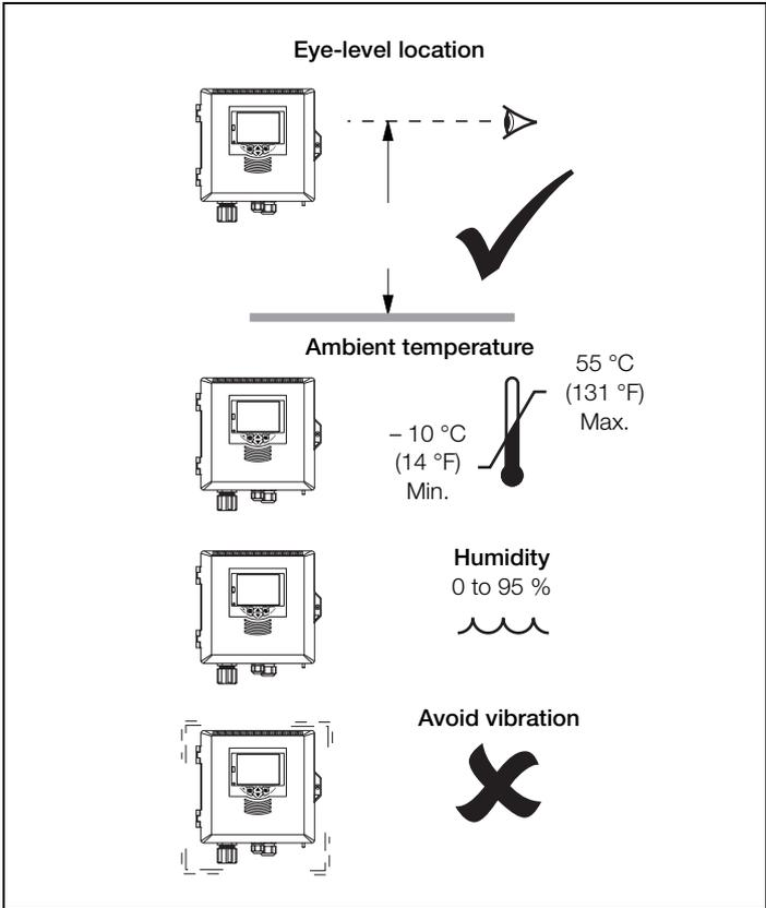
Fig. 1 Transmitter location
