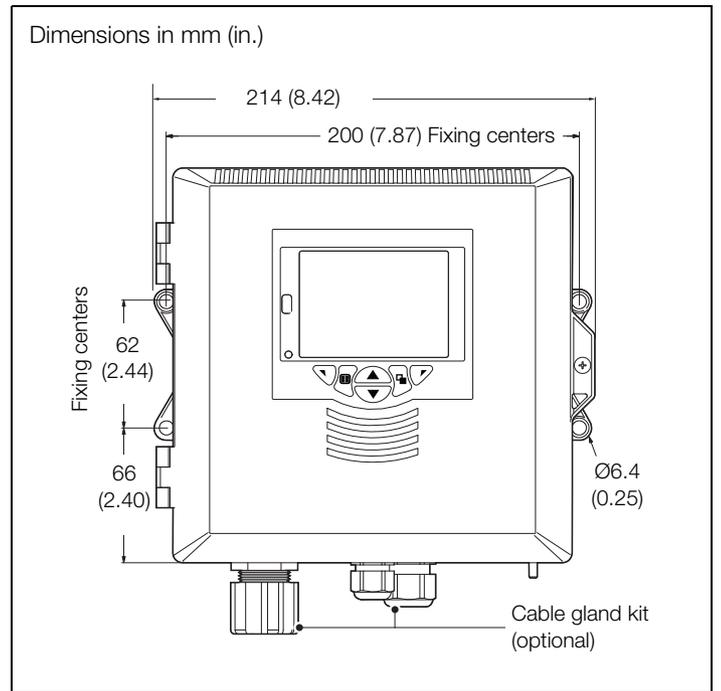
Fig. 4 Transmitter wall-mount option
