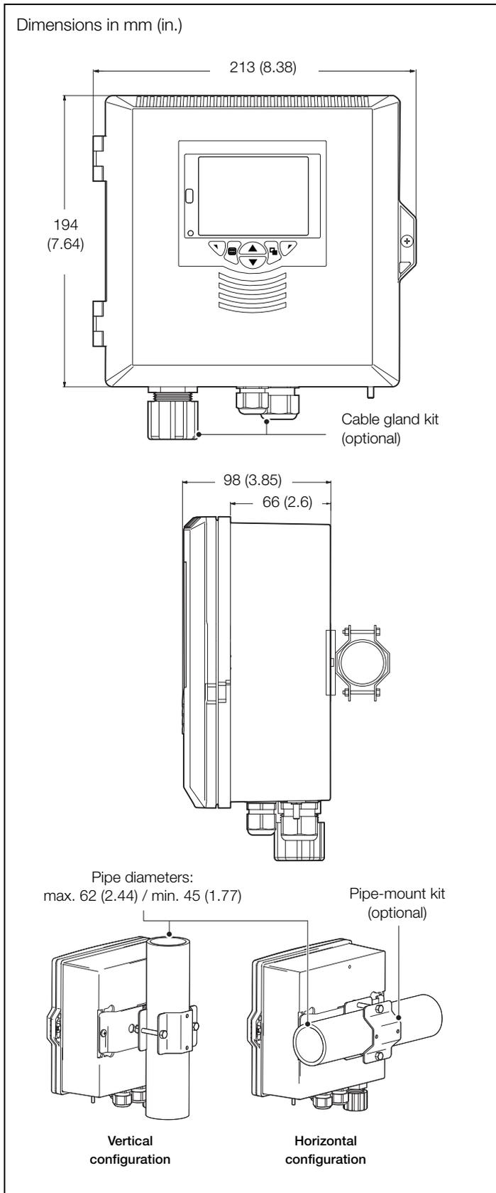
Fig. 3 Transmitter pipe-mount options
