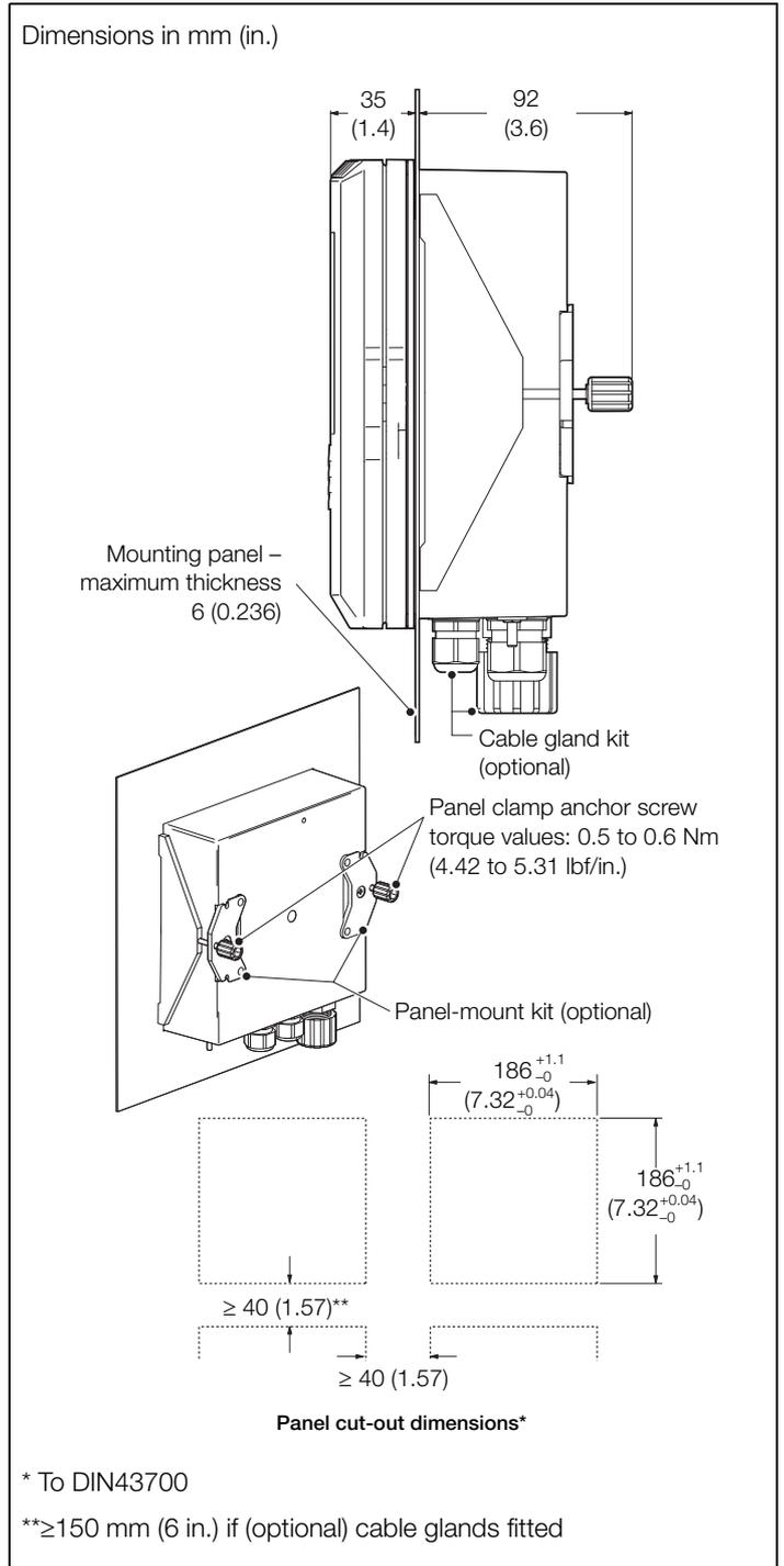
Fig. 2 Transmitter panel-mount option
