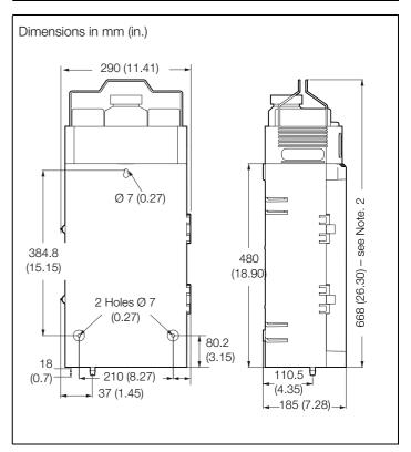
Fig. 2 Sodium wet-section dimensions
