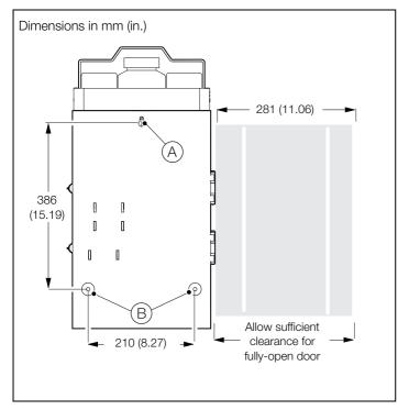
Fig. 3 Mounting the wet-section
