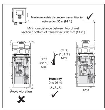
Fig. 1 Locating the wet-section
