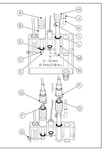
Fig. 5 Fitting the sodium and reference electrodes
