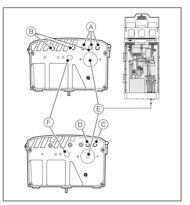
Fig. 4 Connecting the external sample lines and drains
