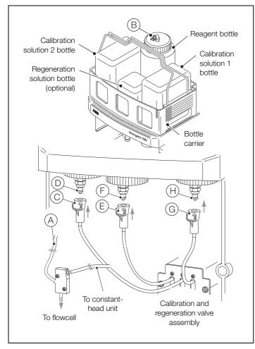
Fig. 6 Reagent, calibration and (optional) regeneration tubing connections
