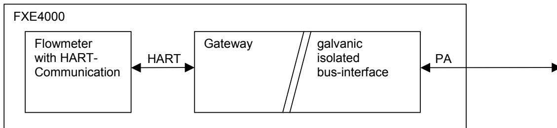
The gateway requires both power supplies being active, the flowmeter supply and the PA BUS supply.
