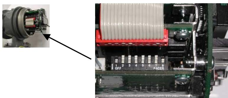
Switch 8 defines whether the address needs to be adjusted via bus or hardware:
