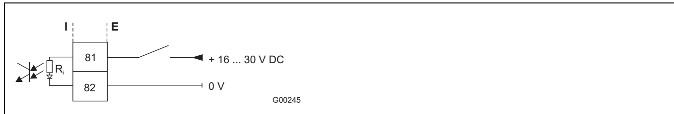
Fig. 34: Contact input for external totalizer reset and external zero return
