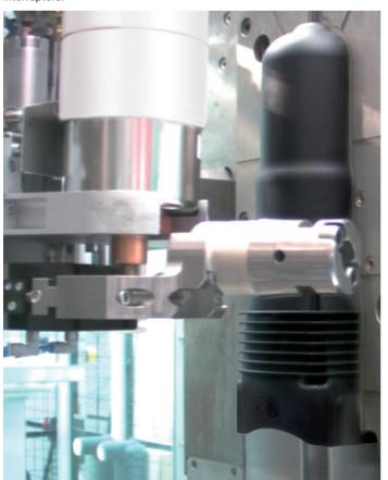
Using a special casting technology, the vacuum interrupter is directly embedded. The maintenance-free vacuum interrupter thus forms a solid unit together with the complete pole.
