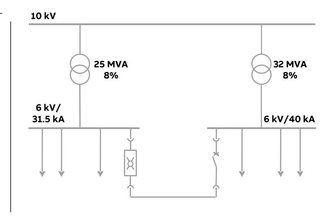
Application: I<sub>s</sub>-limiter in generator feeder
