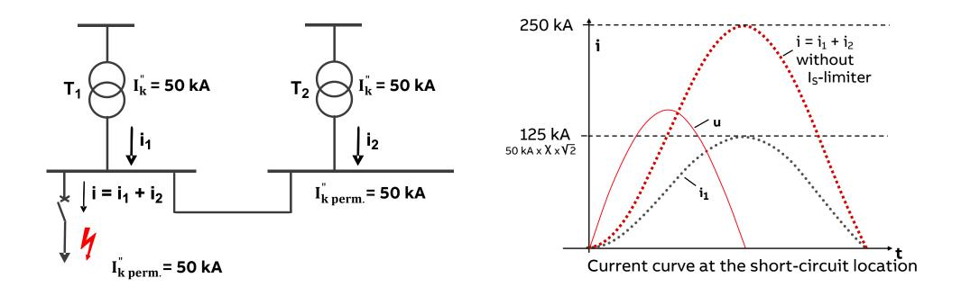
Breaking of a short-circuit current with I<sub>s</sub>-limiter
