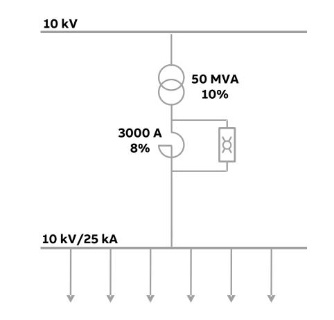
Application: Connection of a generator to a Network with current-direction comparison
