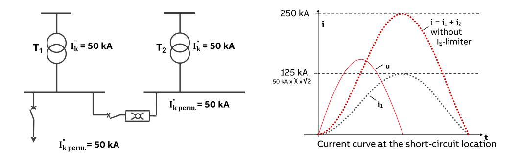
Breaking of a short-circuit current with I<sub>s</sub>-limiter
