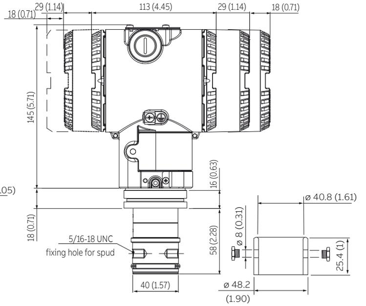
Figure 39 266HRH / 266NRH with barrel housing and direct mount seal S26KN pulp and paper 1 1/2 in. sealing with gasket
