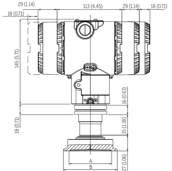
Figure 25 266HRH / 266NRH with barrel housing and direct mount seal S26SS Triclamp (For dimensions of S26 seals refer to the S26 datasheet)
