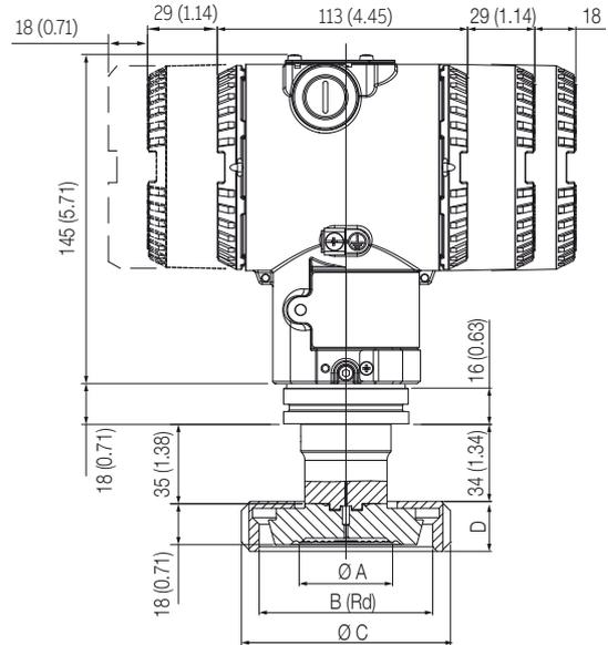
Figure 23 266HRH / 266NRH with barrel housing and direct mount seal S26SS Union Nut (For dimensions of S26 seals refer to the S26 datasheet)
