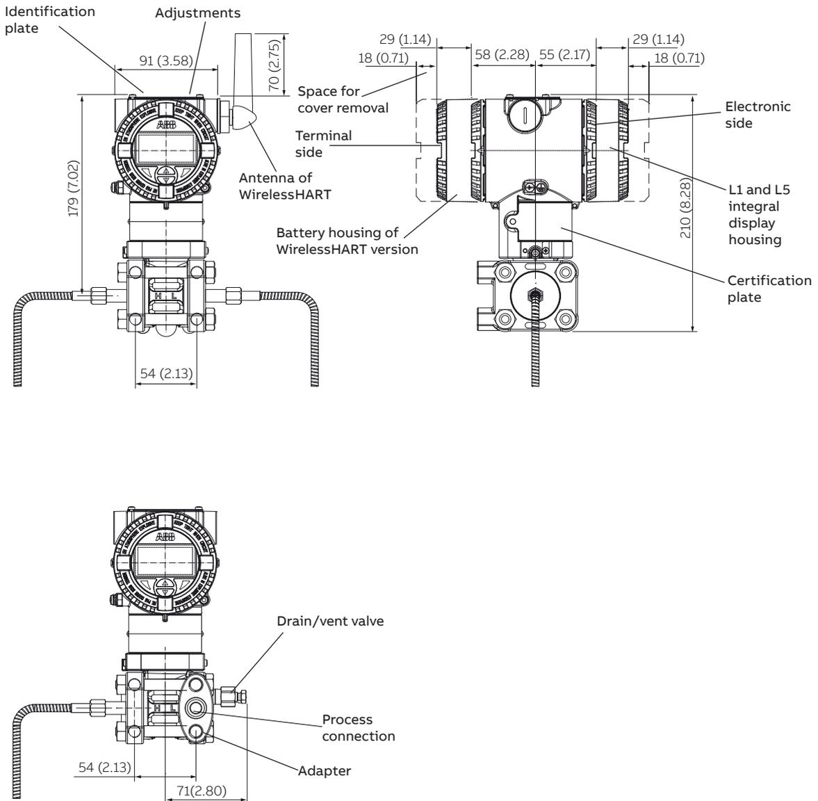
Figure 2 266DRH with barrel housing and remote seal(s)
