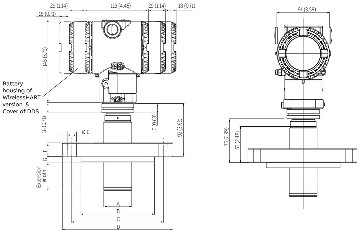
Figure 11 266HRH/266NRH with barrel housing and direct mount seal S26RA/S26RE/S26RJ flanged Raised Face extended diaphragm (For dimensions of S26 seals refer to the S26 datasheet)
