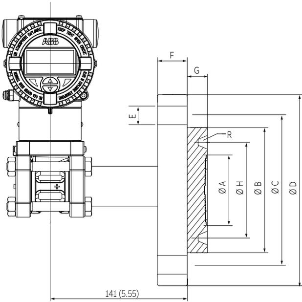
Figure 12 266DRH with barrel housing and direct mount seal S26RR flanged Ring Joint flush diaphragm (For dimensions of S26 seals refer to the S26 datasheet)
