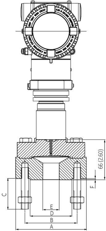
Figure 19 266HRH / 266NRH with barrel housing and direct mount seal S26Mx off-line flanged (For dimensions of S26 seals refer to the S26 datasheet)
