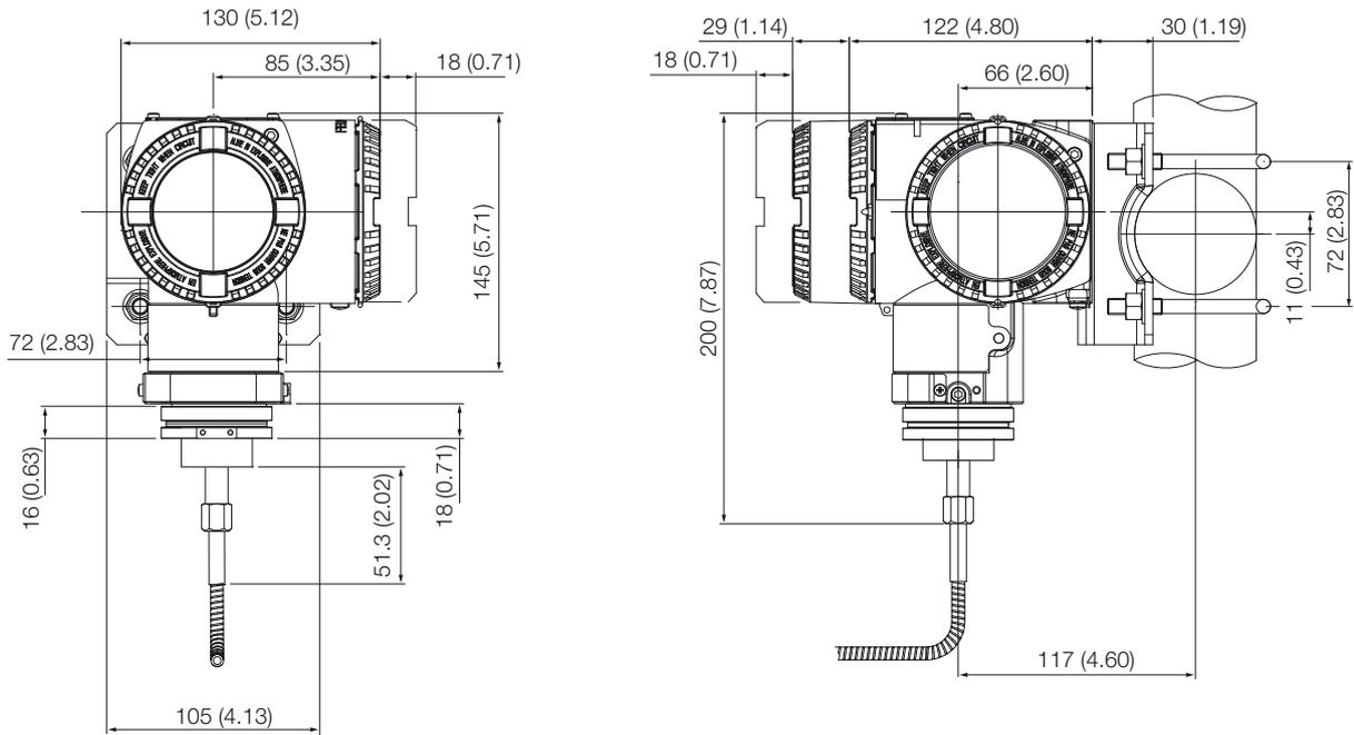
Figure 8 266HRH, 266NRH with DIN housing and remote seal(s) on bracket for vertical or horizontal 60 mm. (2 in.) pipe sensors F, H, M, P, Q, S, W
