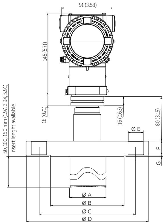
**Figure 16** 266HRH/266NRH with barrel housing and direct mount seal S26FA/S26FE fixed flange Raised Face ASME and EN 1092/1 smooth and Form B1; S26FE Form E (extension not available). (For dimensions of S26 seals refer to the S26 datasheet)
