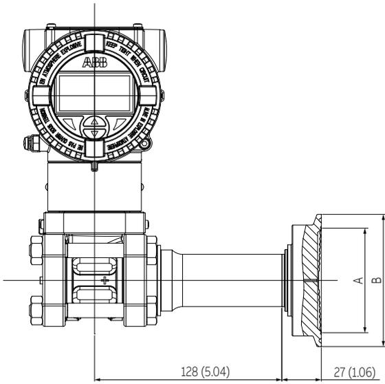
Figure 24 266DRH with barrel housing and direct mount seal S26SS Triclamp (For dimensions of S26 seals refer to the S26 datasheet)
