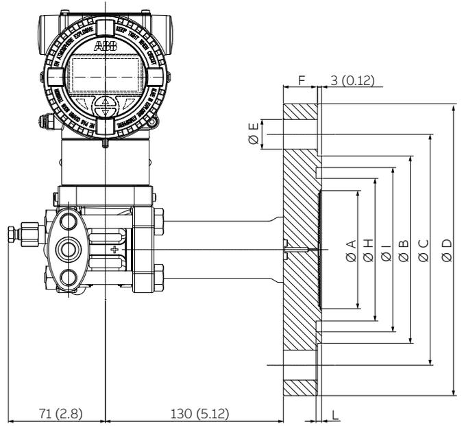
**Figure 14** 266DRH with barrel housing and direct mount seal S26FA/S26FE fixed flange Raised Face flush diaphragm ASME and EN 1092/1 smooth and Form B1 (flushing ring as option, only for flush version); Form E (For dimensions of S26 seals refer to the S26 datasheet)
