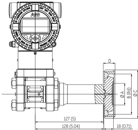
Figure 22 266DRH with barrel housing and direct mount seal S26SS Union Nut (For dimensions of S26 seals refer to the S26 datasheet)
