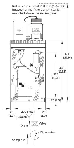
Maximum distance between sensing panel and transmitter 10 m (32.8 ft.) (with detachable-cable electrode option).
