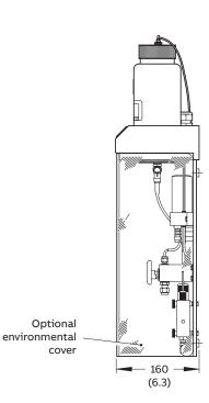
**Note.** 160 mm (6.29 in.) space required below the sensor panel to allow for the opening of the optional environmental cover.
