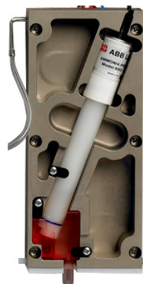
Figure 3 Electrode in temperature-controlled flow cell
