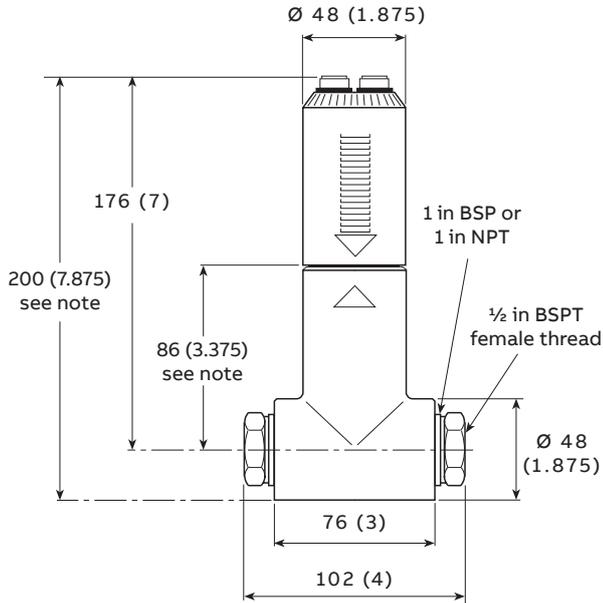
**Note.** Allow an additional 130 mm (5.125 in) for connectors and cartridge removal.
