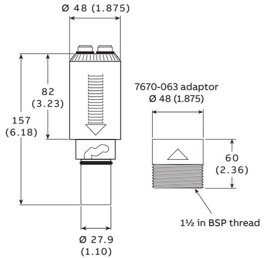
Bayonet cartridge with 7670-063 pipeline adaptor
