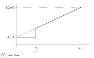
Figure 15: Behavior of the current output
