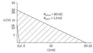
Figure 18: Range of the external supply voltage and current
