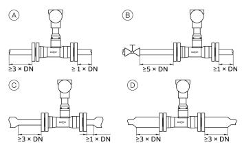
Figure 7: Straight pipe sections
