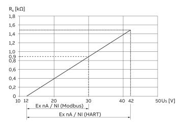
The voltage  $U_S$  = 12 V is based on a load of 0  $\Omega$ .
