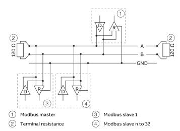
Figure 20: Modbus network (example)
