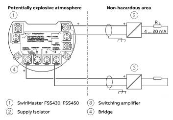
Figure 24: Electrical connection (example)
