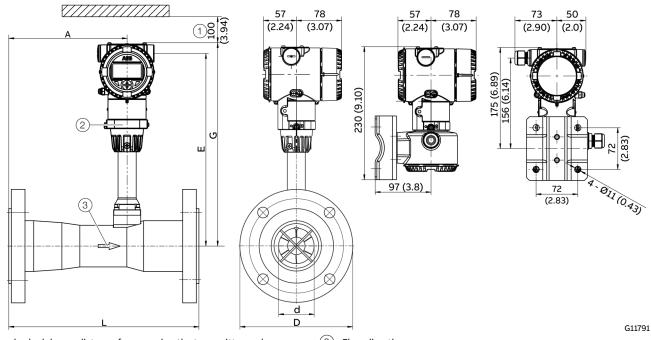
Required minimum distance for removing the transmitter and disassembling the sensor unit
