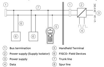
Figure 25: FISCO Control drawing (example)
