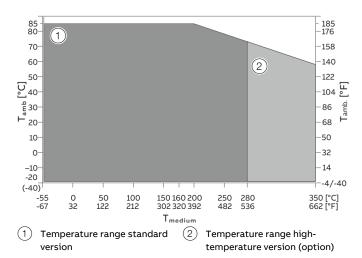
Figure 4: Measuring medium temperature  $\mathbf{T}_{\text{medium}}$  dependent on the ambient temperature  $\mathbf{T}_{\text{amb.}}$
