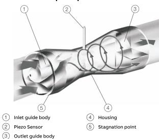
Figure 2: Measuring principle
