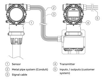
Figure 23: Signal cable installation with FM/CSA
