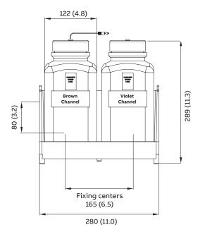
Figure 7 Reagent bottles mounted on optional bracket
