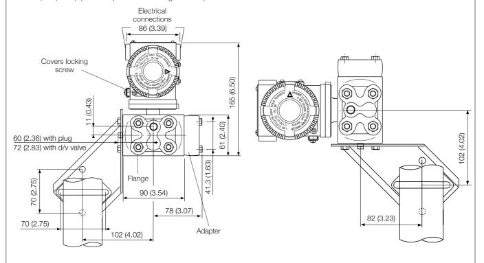
NOTE: Process connection, gasket groove and gaskets are in accordance with DIN 19213. Bolting threads for fixing adapter or other devices (i.e. manifold etc.) on process flange is 7/16 - 20 UNF.
