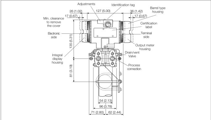
(\*) 51 (2.01), 54 (2.13) or 57 (2.24) mm (in) according to ½ – 14 NPT adapters fitting; 54 (2.13) mm (in) on ¼ – 18 NPT process flange 54 (2.13) mm (in) with low pressure side flange without process connection and drain/vent valve
