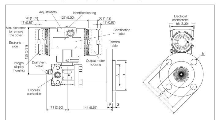
NOTE: Low pressure side opposite to direct mount seal can be a conventional flange or suitable for capillary to remote seal.
