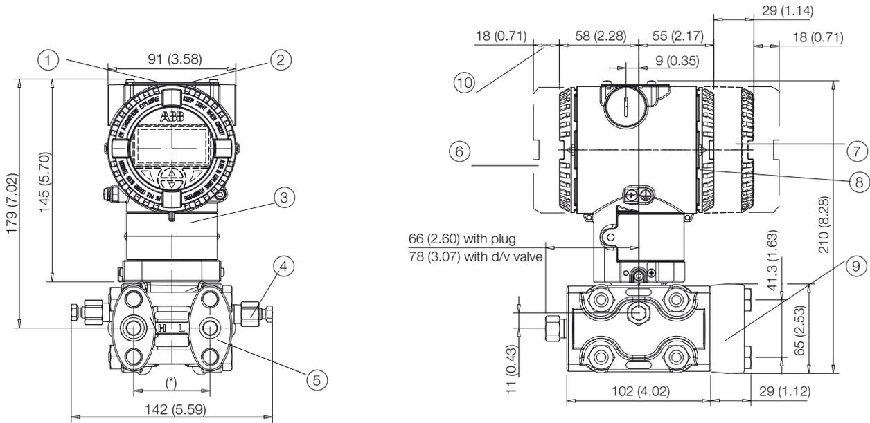
(\*) FOR MODEL 266DSH: 54 (2.13) mm. (in.) on 1/4 in. – 18 NPT process flange; 51 (2.01), 54 (2.13) or 57 (2.24) mm. (in.) according to 1/2 in. – 14 NPT adapters fitting;
