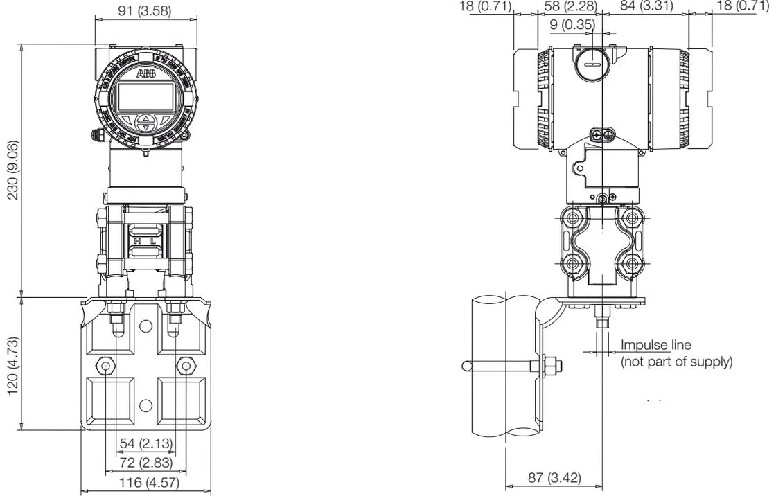
**Transmitter with vertical flanges on flat bracket for vertical or horizontal 60 mm. (2 in.) pipe mounting**
