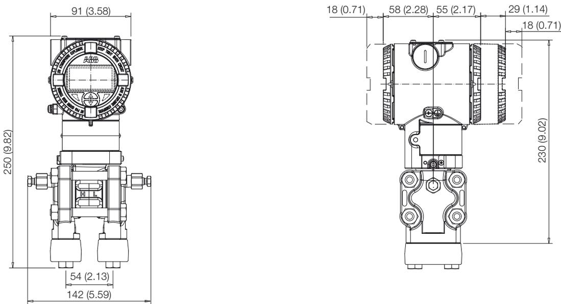
Transmitter on bracket for vertical or horizontal 60 mm. (2 in.) pipe mounting
