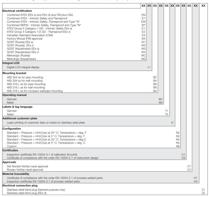
Note 1: Not available with Diaphragm material / Fill fluid code H Note 2: Not available with Diaphragm material / Fill fluid code R
