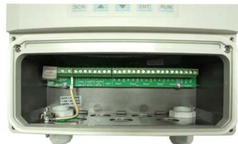
Figure 1 Terminal access on the LST400
