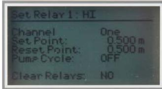
When it is important to keep the loads to the pump balanced we can use pump cycling. If the same pump always switches on first and then switches off last, it will carry a much larger load than any of the other pumps. This will mean earlier need for maintenance on this first pump. At the same time the other pumps will be underutilized. LST400 has two different modes to ensure the running time of the pumps is balanced. These are referred to as First In First Out (FIFO) and Rotate Pump Cycling.
