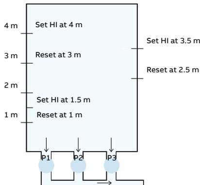
Figure 2 Example of a pump cycling system
