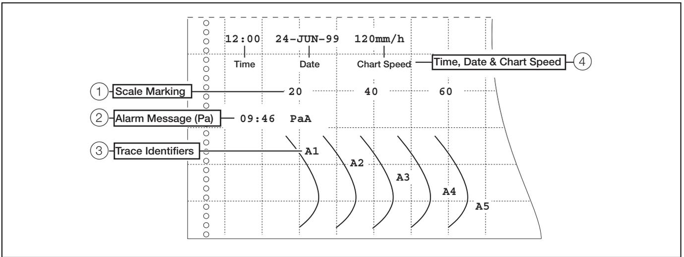
① **Scale Marking** – one scale per trace, printed across the width of the zone, at intervals of 20 to 240 mm.
